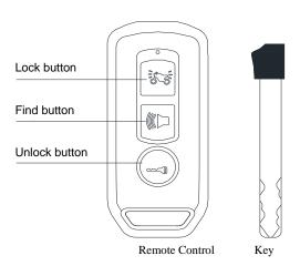
Unlock button: press the Unlock button to exit alert mode.
