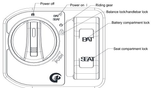
**Power off:** when the knob is turned to the upright position, the motorcycle's power is turned off, and the key can be removed.
